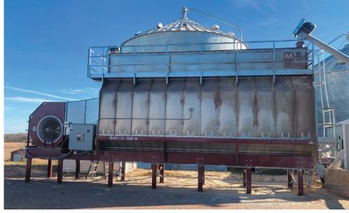
Bill Delander of Roberts, Wisconsin was looking to upgrade his dryer to a newer dryer with more drying capacity and new technology. Bill went with an MC 600 Eco continuous flow dryer. This dryer has a 30hp low speed centrifugal fan for quiet drying, aluminum outer screens, a dual 20/ 20 pinnacle touch screen controller, MC Trax for remote monitoring, and Accu-Dry and Tru-Dry automatic moisture control drving.
