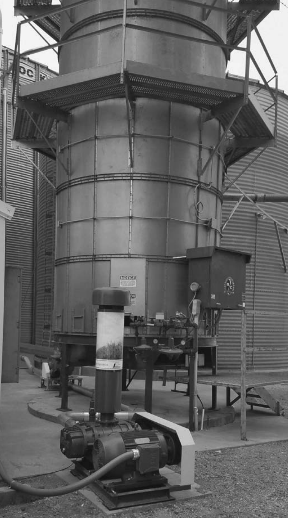
Steve Carlson Steve Carlson of Welch, MN purchased a new Jemco Vari-Air grain transfer system. The new Vari-Air has a tri-lobe blower that is very quiet and a Jemco control panel for ease of operation. The corn is transferred through 5" piping held together with four-bolt compression couplers and is dumped into the bins through large cyclones with liners.
