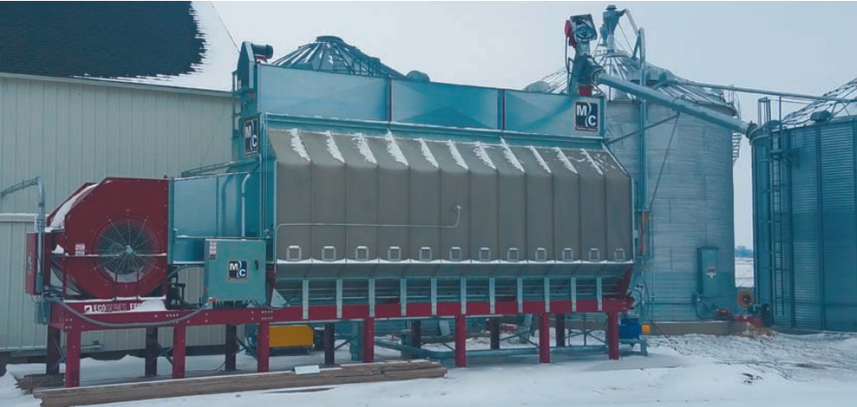
Chris Kalass Chris Kalass of Goodhue wanted to become more efficient with his grain drying. After some discussion with our sales staff he chose to install a new MC EcoSeries E600 grain dryer. The dryer is single phase with twin 15hp motors and a very quiet belt driven centrifugal blower. The dryer has a Pinnacle 20/20 touch screen control with remote control and features TruDry moisture control with a DM510 sensor. Chris also purchased a new Jemco VariAir grain conveying system with a 30hp motor. Chris has single phase power so the VFD converts the power for him. The air system has large cyclones and bin consigner.
