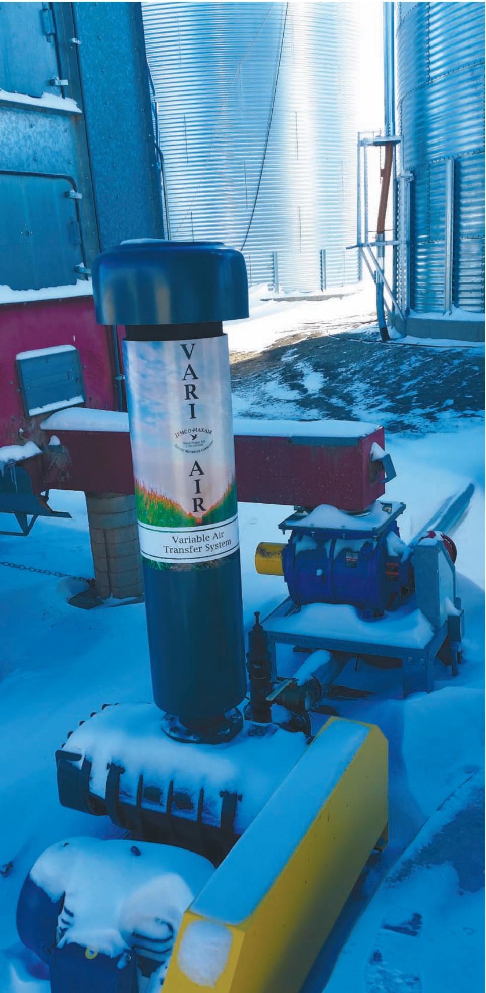
Bruce Olson Bruce Olson of Vasa was looking to upgrade his drying system and get rid of his takeaway dry augers. He contacted Lodermeier’s and we came up with a solution to upgrade to a 5” Jemco air system. The system has a 20hp motor on the blower, controlled by a VFD to regulate the speed of the grain in the system. It has an air lock under the discharge of the dryer and a selector valve mounted to the bin wall to fill multiple bins.
