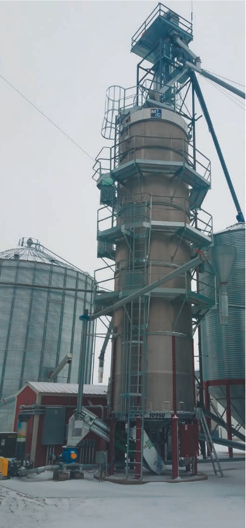
Steve Carlson Steve Carlson of Welch decided to replace his existing MC grain dryer. After some careful planning he purchased a new MC 10950 continuous flow tower dryer. The dryer features a very quiet inline centrifugal blower and a Midco burner. The dryer has aluminum outer screens. A new Pinnacle 20/20 touchscreen controls the dryer temperature and the DryerMaster moisture control system. The MC Trax gives Steve the capability of controlling and monitoring the dryer when away from the grain setup. To accommodate the taller dryer our crews raised the tower and leg. After the dryer was put in place a new Sukup grain pump was installed under the dryer to take the corn to the Jemco air system.
