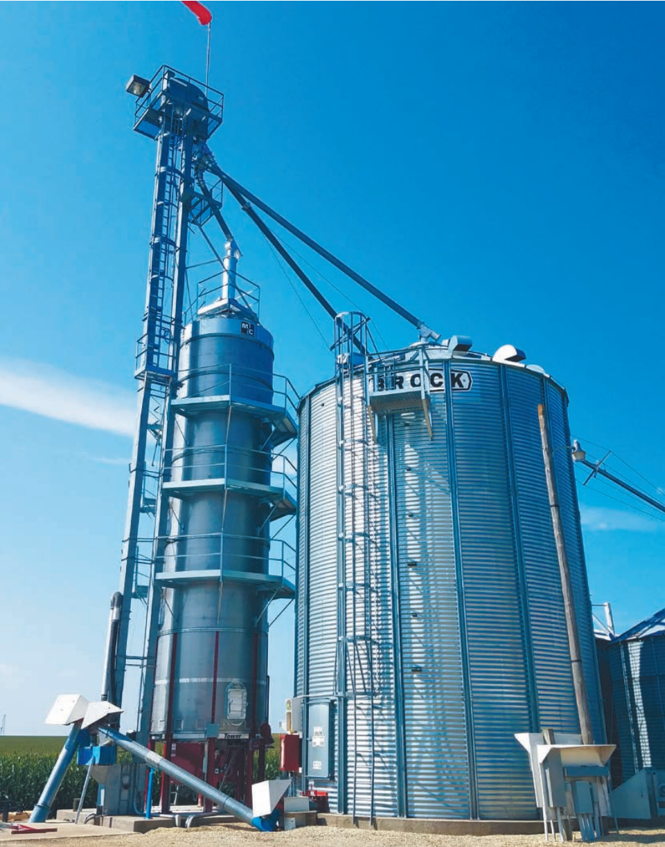
Tom Nelson Tom Nelson of Cannon Falls decided to upgrade his MC dryer for some new technology. Tom purchased a new MC 10950 continuous flow tower dryer. The tower has a vacuum cool/pressure heat method of drying for a very efficient dryer. The dryer has stainless steel outer screens with three outer service catwalks. MC 20/20 controls and the MC Trax monitoring with remote control enables Tom to keep good track of the AccuDry moisture system.
