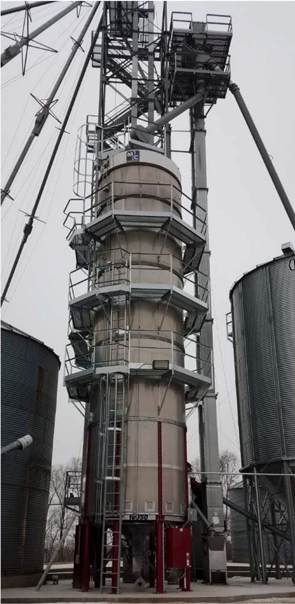
Tom Goebel Tom Goebel of Cottage Grove decided it was time to update his grain dryer. He worked with Lodermeier’s and went with an MC 10950 tower dryer. The dryer showed up in modular sections and worked for fast and easy installation. Some features on the dryer included aluminum outside screens, stainless steel floor, three outside catwalks, Accu-dry moisture controls, and the new Pinnacle 20/20 control system for the dryer.
