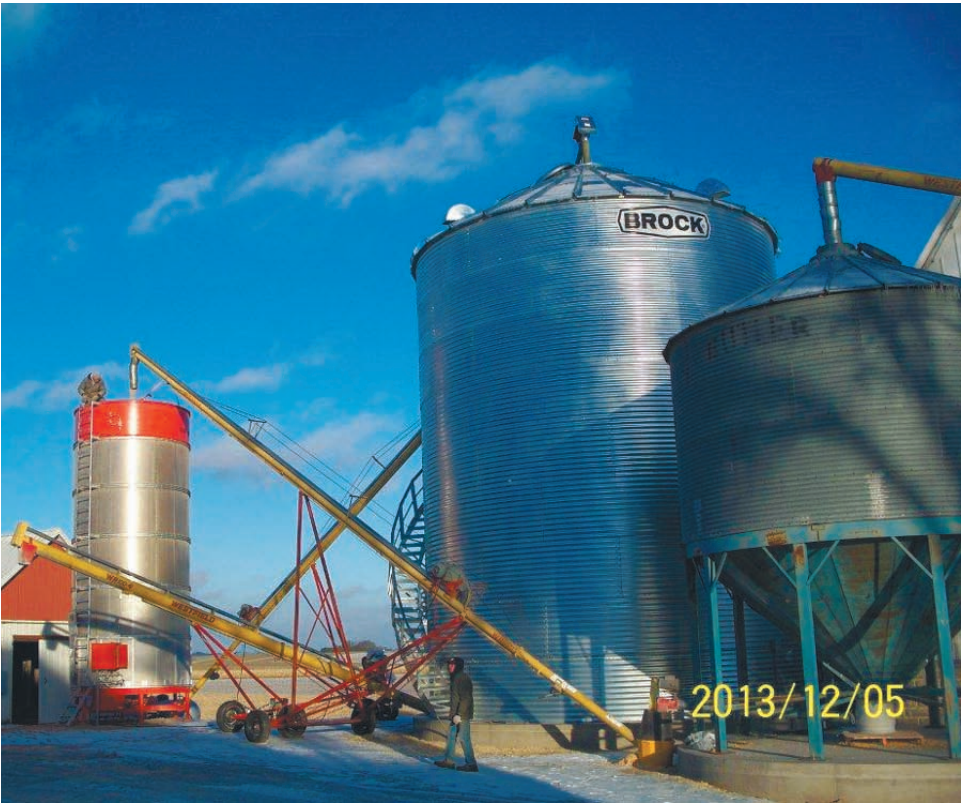
Jon Meyer Jon Meyer of Lake City, MN was looking to add more storage and a faster way to dry grain. Jon purchased from Lodermeier's this Brock 27' x 33' grain bin, with full floor aeration, 8" sweepmaster bin sweep and Brock grain spreader. To increase his drying capacity, Lodermeier's installed this pre-owned Kan-Sun 10-25-215 grain dryer which was refurbished by Lodermeier's.
